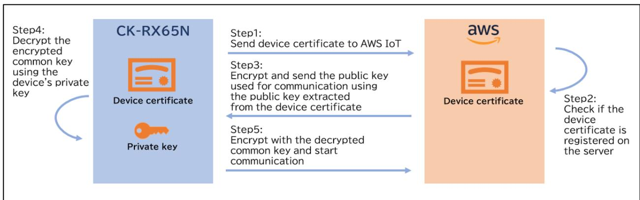
Figure 2.2 IoT Device Provisioning
