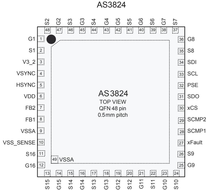
Figure 4.1 : Pin Diagram of AS3824 (Top View)
