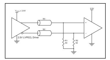
Figure 8C. 2.5V LVPECL Driver Termination Example
