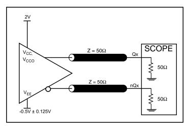
2.5V Core/2.5V LVPECL Output Load AC Test Circuit
