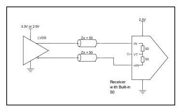
Figure 5A. IN/nIN Input with Built-In 50 $\Omega$  Driven by an LVDS Driver
