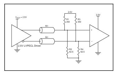
Figure 8A. 2.5V LVPECL Driver Termination Example
