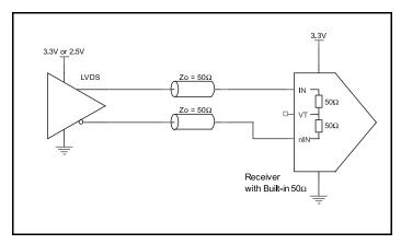
Figure 4A. IN/nIN Input with Built-In 50 $\Omega$  Driven by an LVDS Driver
