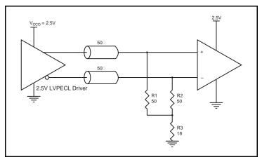
Figure 8B. 2.5V LVPECL Driver Termination Example
