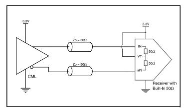
Figure 4C. IN/nIN Input with Built-In 50 $\Omega$  Driven by a CML Driver
