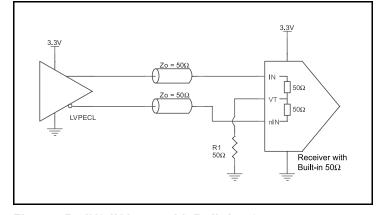
Figure 4B. IN/nIN Input with Built-In 50 $\Omega$  Driven by an LVPECL Driver
