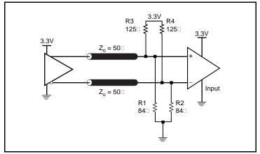
Figure 7A. 3.3V LVPECL Output Termination
