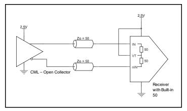
Figure 5C. IN/nIN Input with Built-In 50 $\Omega$  Driven by a CML Driver
