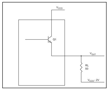
Figure 9. LVPECL Driver Circuit and Termination
