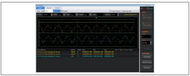
Figure 12-1 Waveforms in the State Where the Voltage is Rising Up to 390 V under PFC Control
