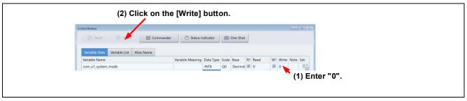
Figure 6-6 Procedure for Stopping the Motor
