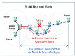
Wi-SUN FAN has been deployed in millions of smart meters worldwide and has great potential also for smart cities and smart grids for applications such as smart homes, building management, and lighting systems.
