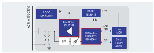
Note: Serial flash memory is not required when the firmware is downloaded from the host MCU.
