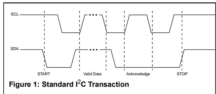
**Figure 1: Standard I<sup>2</sup>C Transaction**
