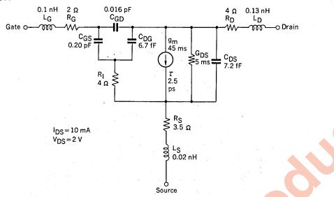
Note: Inductance of bonding wires are included.
