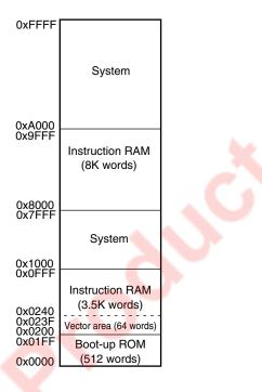
Caution Programs and data cannot be placed at addresses reserved for the system, nor can these addresses be accessed. If these addresses are accessed, the normal operation of the device cannot be guaranteed.
