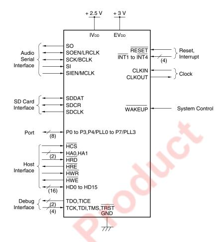
**Remark** The P4 to P7 pins are multiplexed with PLL0 to PLL3 pins.
