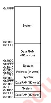
Caution Programs and data cannot be placed at addresses reserved for the system, nor can these addresses be accessed. If these addresses are accessed, the normal operation of the device cannot be guaranteed.
