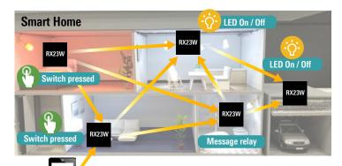
Perform initial settings to build a mesh network and switch the LED on/off easily with a smartphone.
