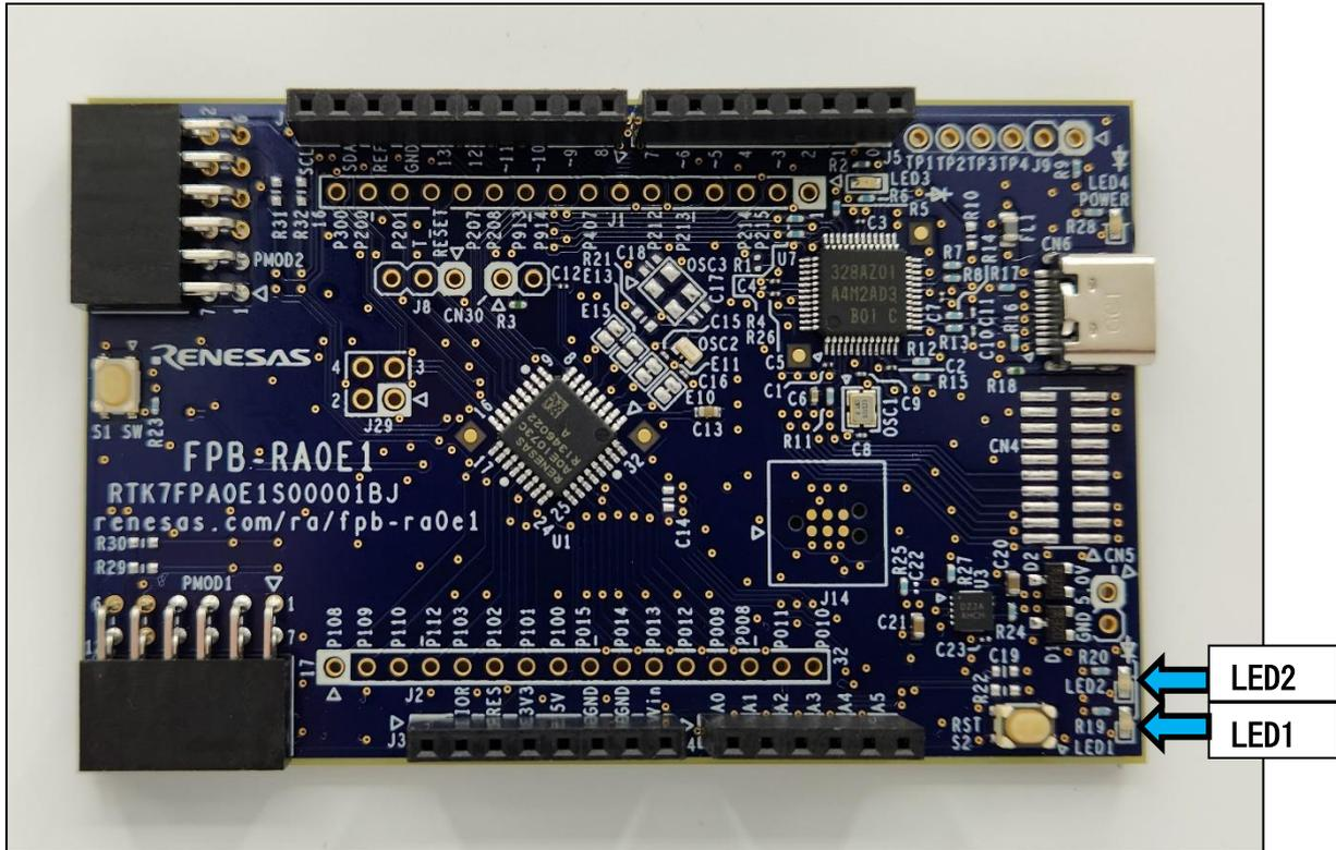
Figure 2-1 On-board LED position
