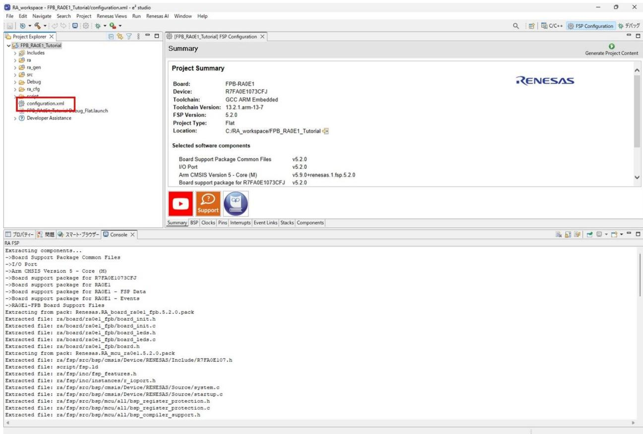
Figure 3-13 How to call the FSP Configurator screen
