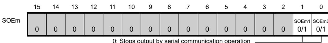
\* For channel n, whose serial output is stopped, the SO<sub>m</sub>n bit value of the SOm register can be set by software.
