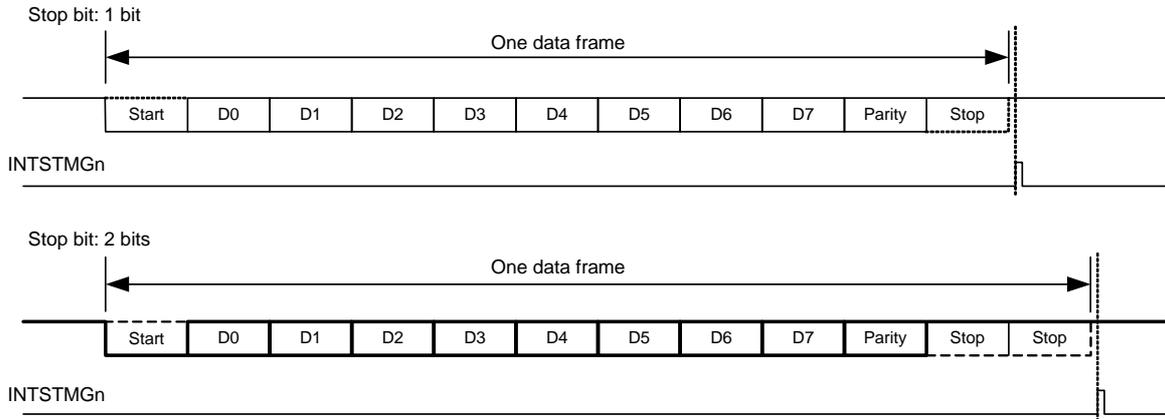
(2) When ISSMMGn = 1 (Transmit buffer empty interrupt)
