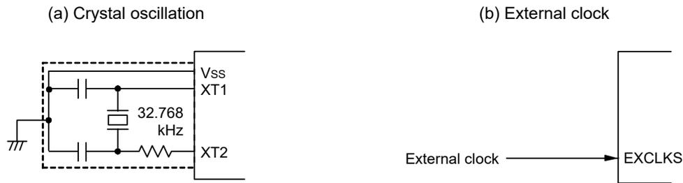
**Caution** When using the X1 oscillator and XT1 oscillator, wire as follows in the area enclosed by the broken lines in the Figures 6-20 and 6-21 to avoid an adverse effect from wiring capacitance.
