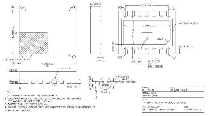
Figure 3. 14-Lead TDFN Package
