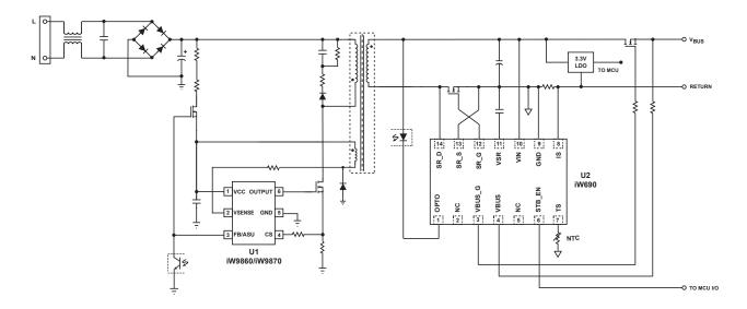
Figure 1. iW690 Typical Application Circuit for Multi-Level Voltage and Current (Using iW9860/iW9870 as Primary-Side Controller, Achieving < 5mW No-Load Power Consumption).
