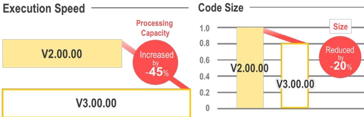
(Note): The comparative tests were performed on a benchmark program for embedded systems using a same MCU with the same option settings. The improvement will depend on the program used.
