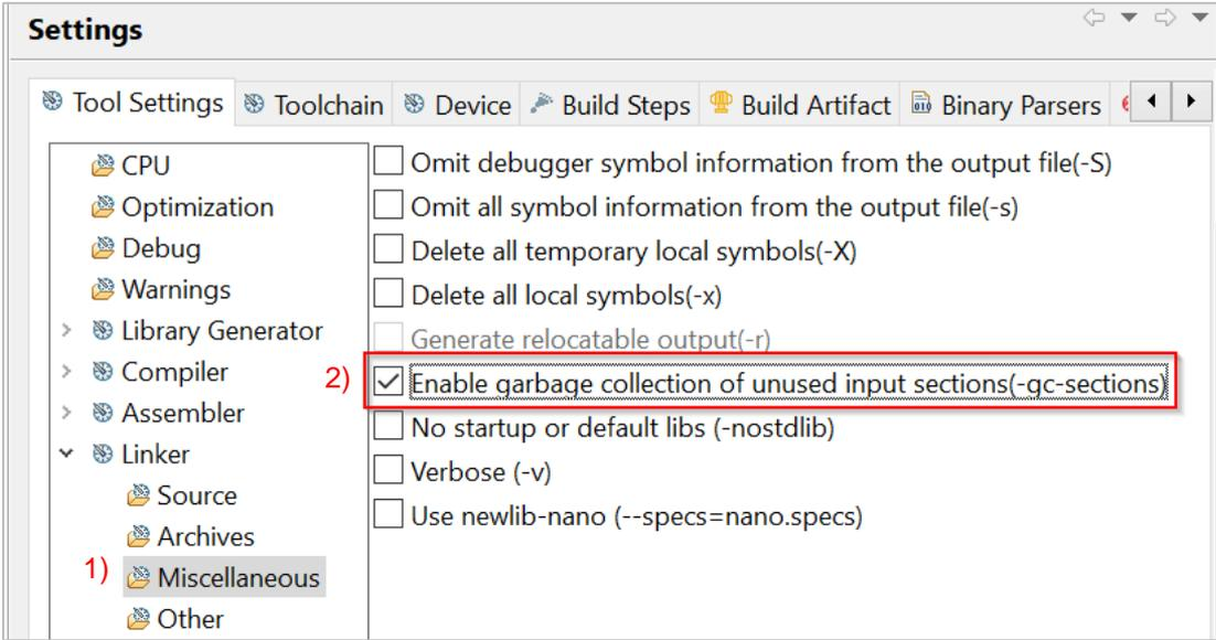
Figure 1 Linker setting for GCC RX
