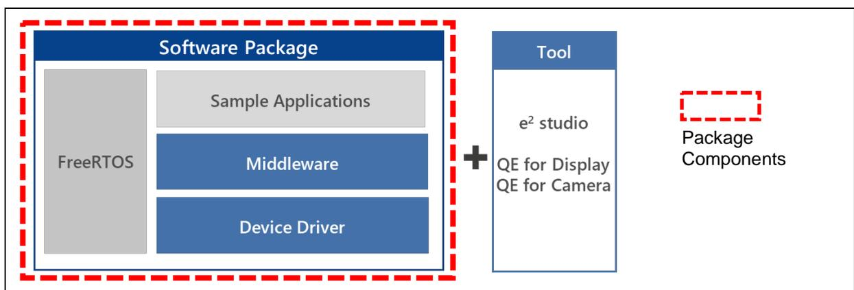
Figure 1 Software Structure of the RZ/A1H Software Package
