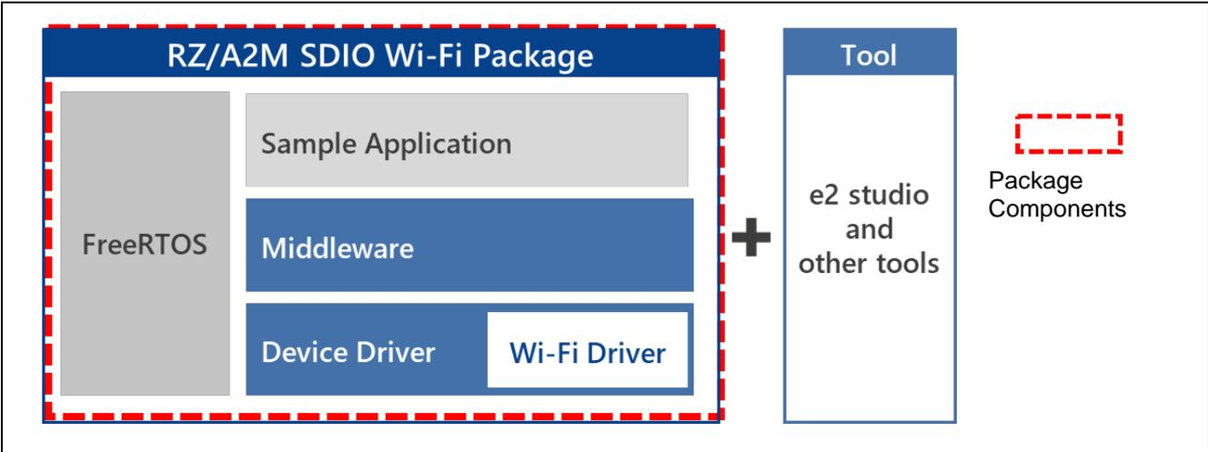
Figure 2 RZ/A2M SDIO Wi-Fi Package Software Structure
