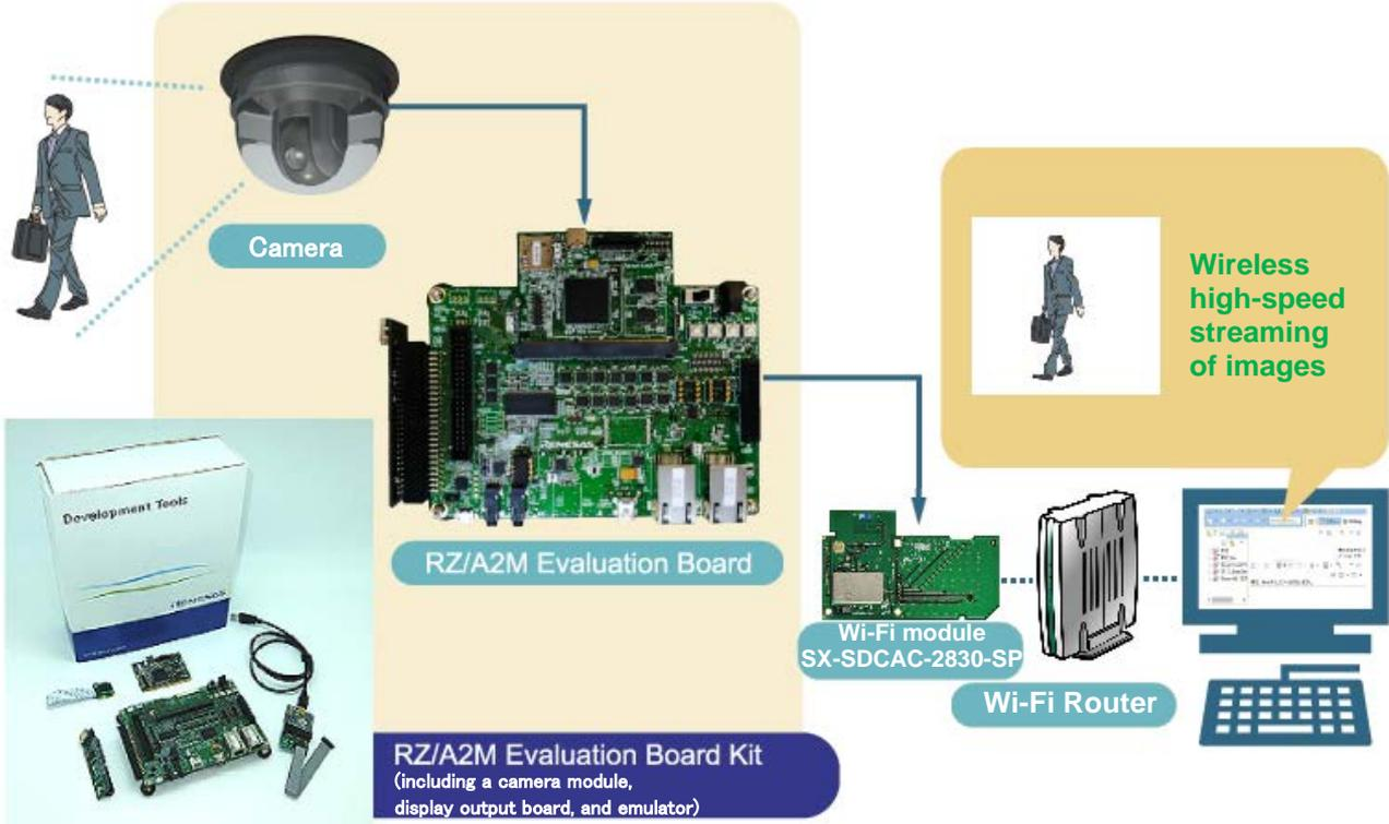
Figure 1 RZ/A2M SDIO Wi-Fi Package Sample Application Image
