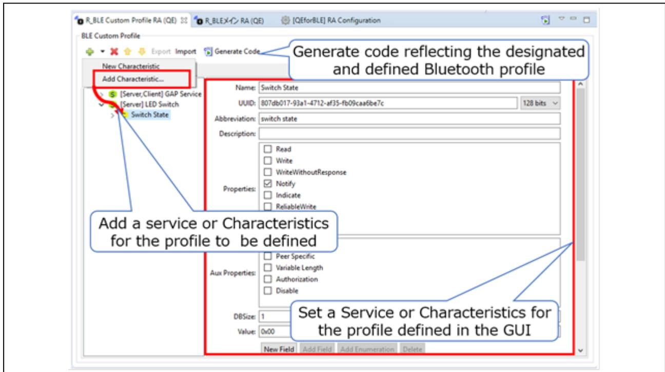
Figure 3 Proprietary Profile Definition and Code Generation
